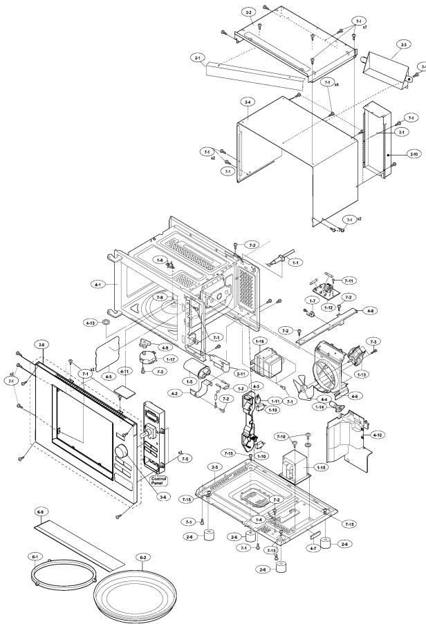
NOTE: In the event of removing the turntable motor cover this part should be refitted using screw connection: 5028 14 53-00/6 (7-10)
